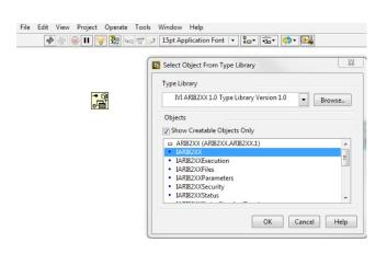
Click OK to finish linking **Automation Open** Block with the **ARI78XX** object.
