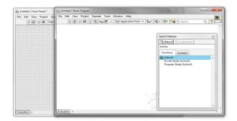
Double Click ActiveX Folder to bring up additional functions under Connectivity. Drag the **Automation Open** function icon onto the block diagram window.
