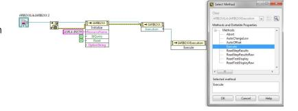
Use the Function Palette to insert a **Close Reference Node**. Next connect the "reference out" of Execution node to "reference" input of the Close Reference node.
